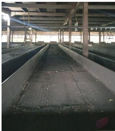
Gambar 39. *Withering Trough (WT)*
