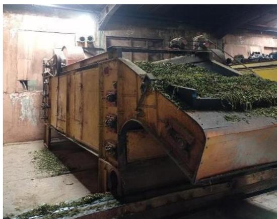
Gambar 43. Mesin *Endeless Chain Pressure* (ECP)
