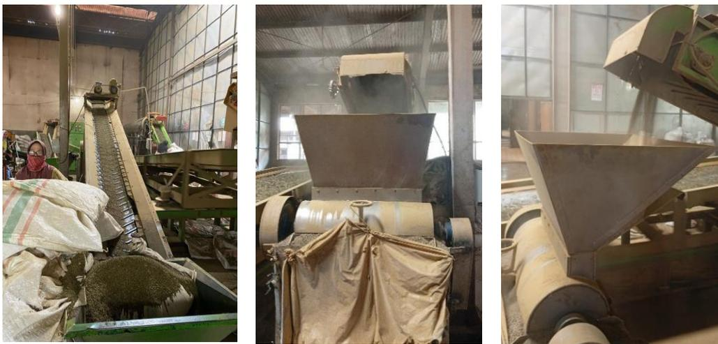
Gambar 51. Mesin *cutter*
