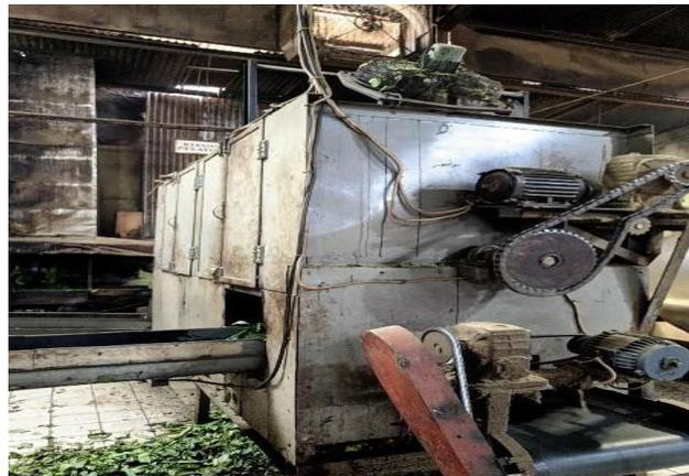
Gambar 41. Mesin *Rotary Cooling*
