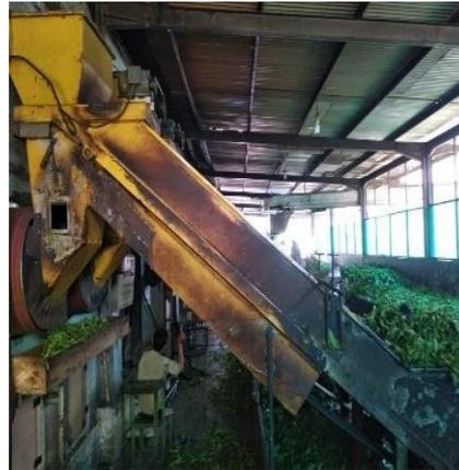
Gambar 40. Mesin *Rotary Panner*
