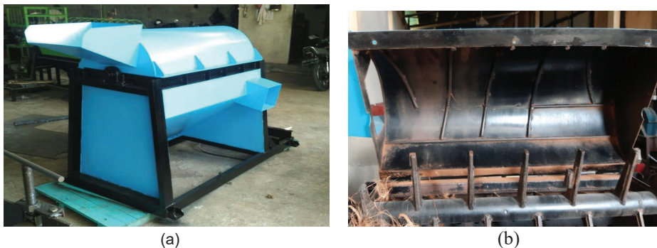
Fig. 6 . The Coconut husk extractor machine, (a) outside, (b) inside
