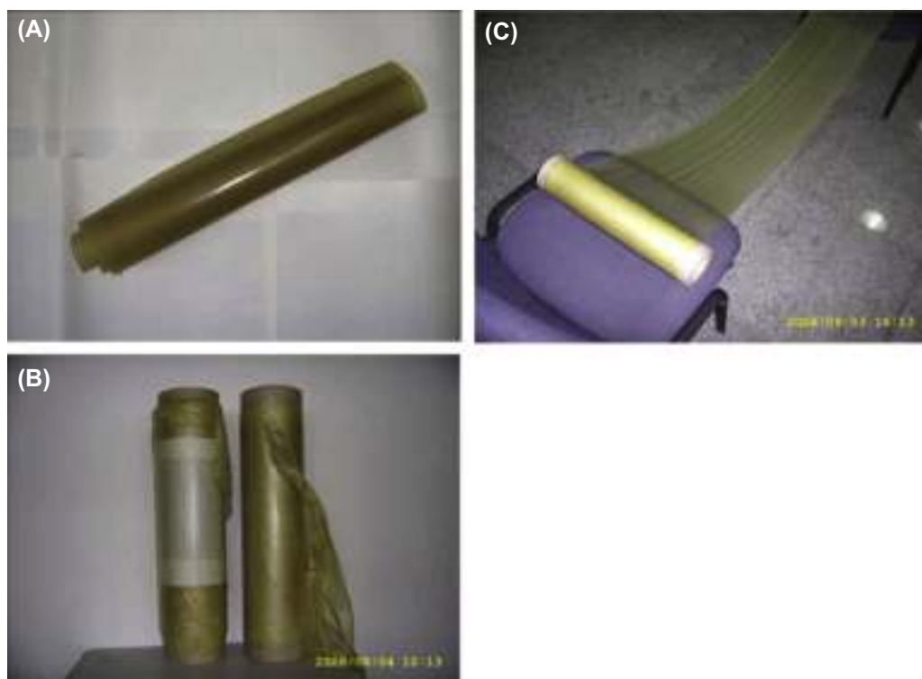
FIG. 8.5 Photographs of CMC/SPI film in expanded and rolled states fabricated by a continuous casting method (Su et al., 2010).
