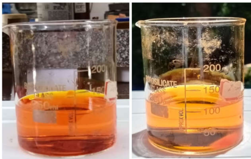
Figure 10. The color intensity before and after photodegradation using green synthesized ZnO nanoparticles.
