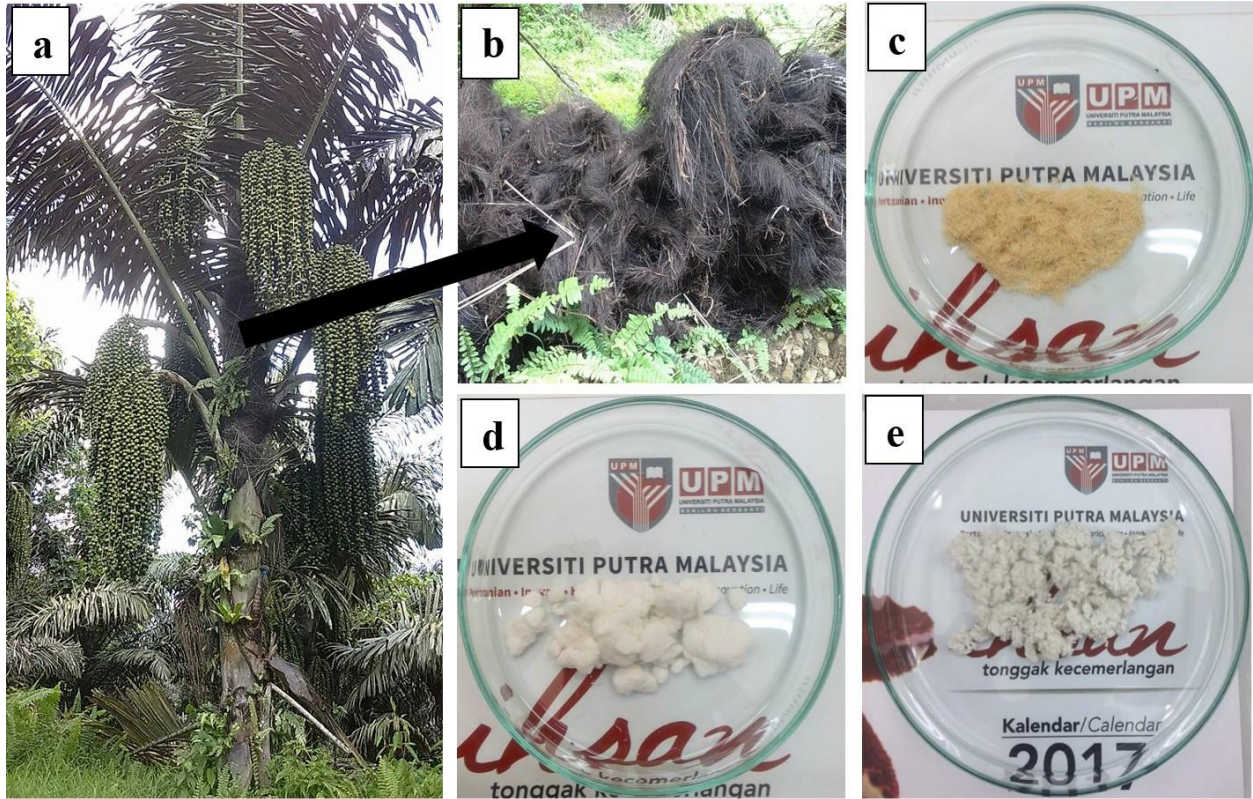
Fig. 1. Photographs of (a) the sugar palm tree, (b) raw sugar palm fibers, (c) bleached fibres, (d) alkali-treated fibres, and (e) refined fibres.
