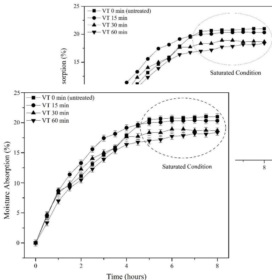
**Figure 4.** Moisture absorption of all tested biocomposite samples. Samples were subjected to ultrasonication for 0, 15, 30, or 60 min. VT: vibration time.
