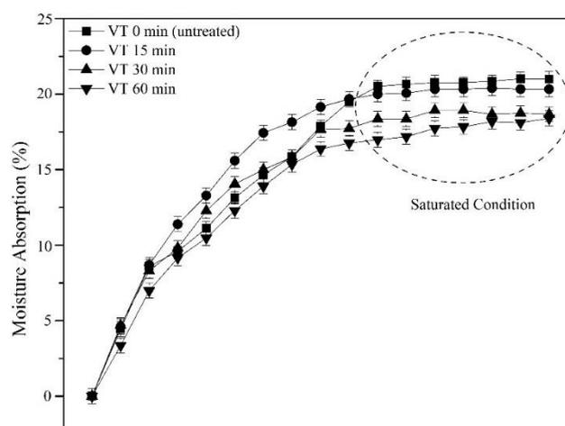
**Figure 4.** Moisture absorption of all tested biocomposite samples. Samples were subjected to ultrasonication for 0, 15, 30, or 60 min. VT: vibration time.
