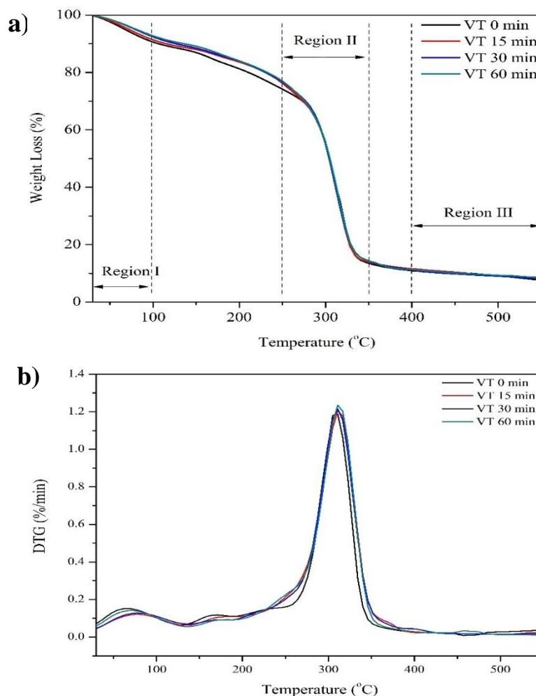
**Figure 3.** (a) Thermogravimetric analysis and (b) DTG curves of all biocomposite samples
