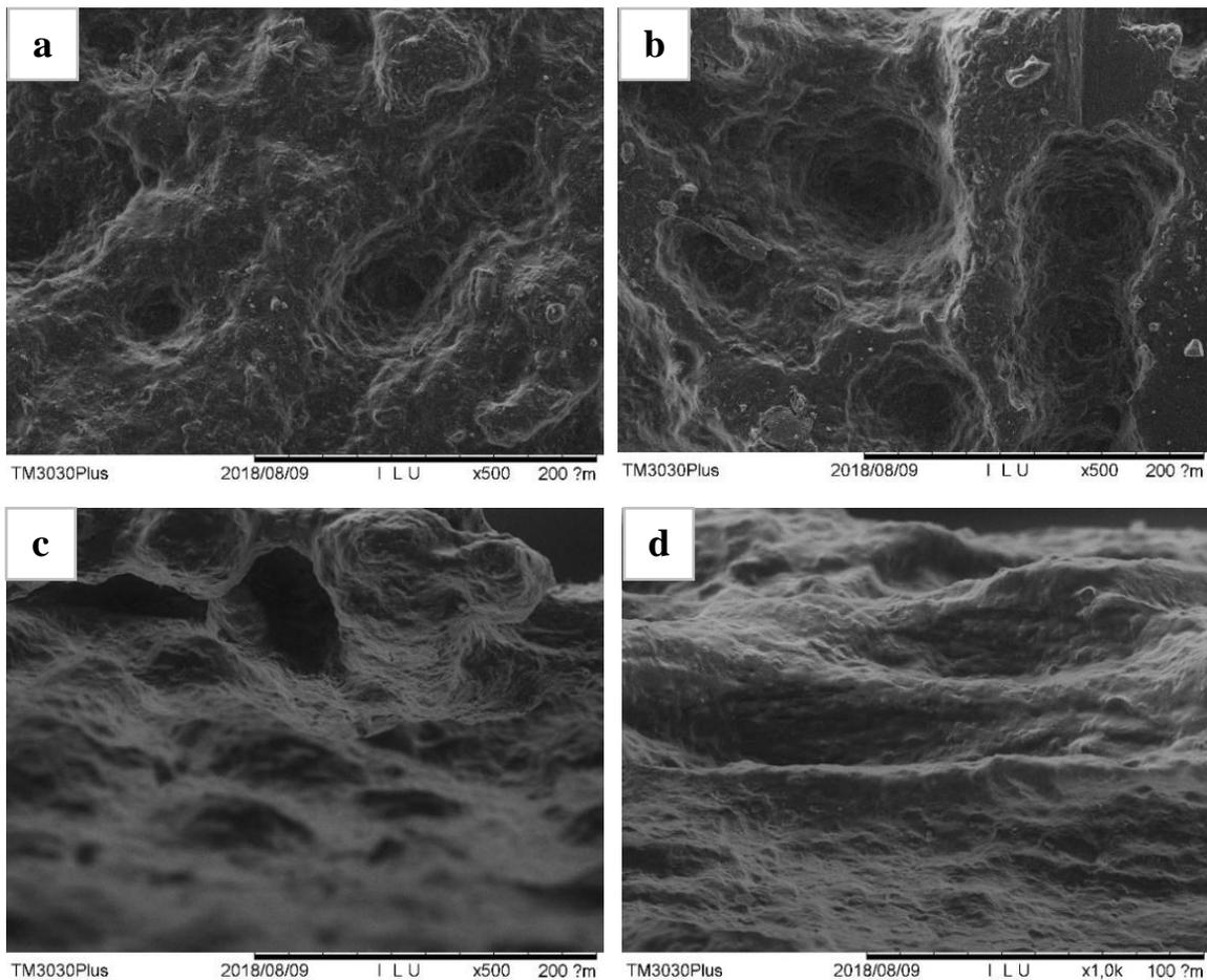
**Figure 7.** Morphological characteristics of biocomposite samples after biodegradation in soil. (a) Untreated (day 3), (b) untreated (day 15), (c) vibrated for 60 min (day 3), and (d) vibrated for 60 min (day 15).
