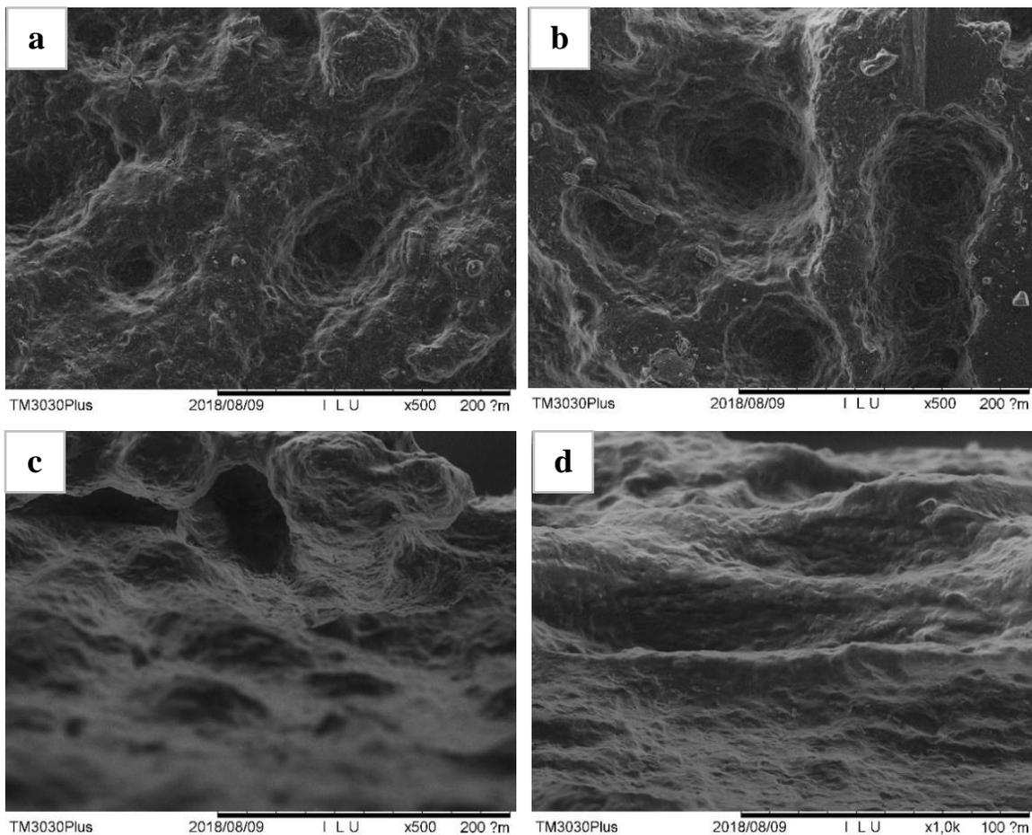
**Figure 7.** Morphological characteristics of biocomposite samples after biodegradation in soil: (a) ~~VT 0 min (3rd Untreated (day 3))~~, (b) ~~VT 0 min (15th untreated (day 15))~~, (c) ~~VT vibrated for 60 min (3rd day) 3)~~, and (d) ~~VT vibrated for 60 min (15th day) 15).~~
