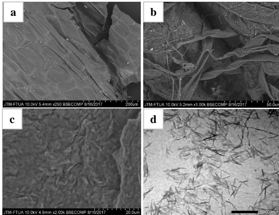
~~FESEM:~~ (a) raw fibreRaw fiber (untreated), (b) bleached fibrefiber, (c) fiber subjected to acid hydrolysis fibre; and ~~using TEM:~~ (d) ultrasonicated fibrefiber subjected to ultrasonication.
