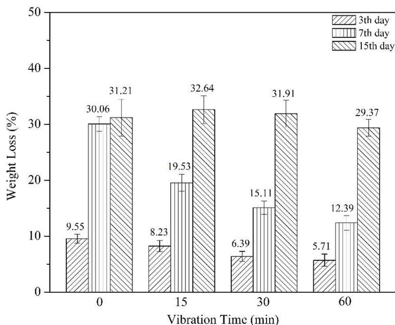
**Figure 6.** Biodegradation rates of all tested biocomposite samples
