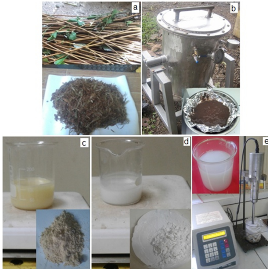
Fig. 2. Synthesis of CNF-ramie process, a) raw, b) pulping ramie, c) Bleaching ramie, d) hydrolysis ramie, e) ultrasonication ramie process.
