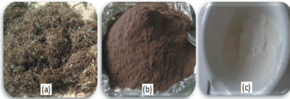
Figure 2. (a) Chopped Ramie fibers, (b) pulped Ramie powder, (c) bleached Ramie powder.
