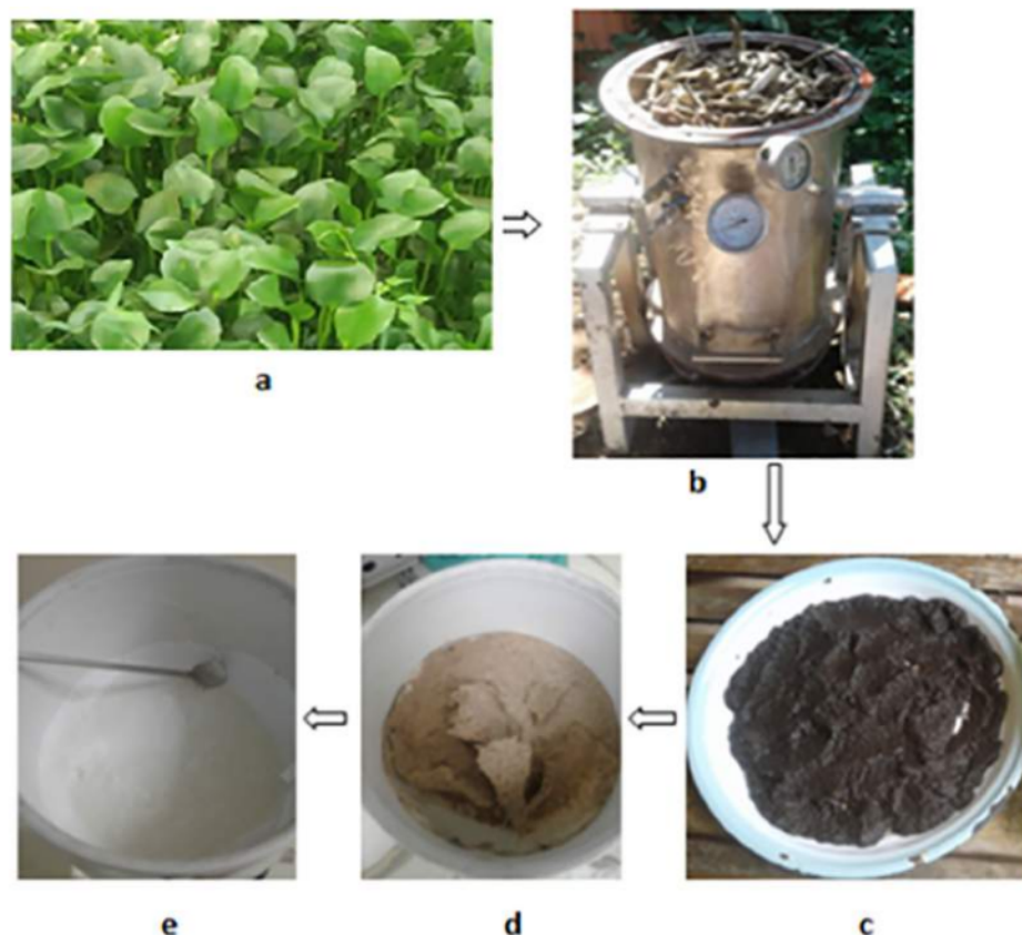
Fig. 1. Isolation process of CMF WH: a) raw WH, b) pulping in digester process, c) pulped WH, d) bleached WH, and e) CMF WH after hydrolysis.
