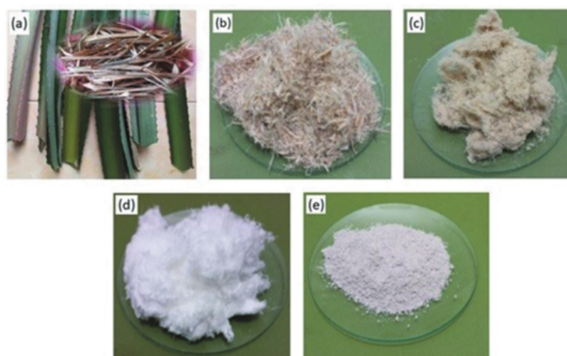
Figure 1. PD fiber leaves (a), dried PD fiber after blending with a blender (b), alkalized PD fiber (c), bleaching PD fiber (d), hydrolyzed PD fiber (e).
