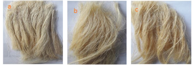
Fig. 3. PFs (a) raw, (b) KOH treated dan (c) NaOH treated.
