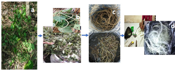
Fig. 1. Paederia foetida , PF, (a) plant, (b) selection of PF stems, (c) Soaking PF in water, (d) Extracting fiber from PF stems.
