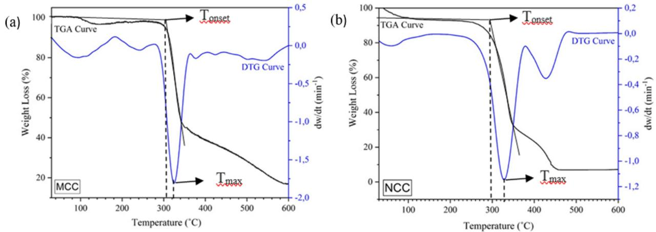
**Figure 6.** TGA and DTG curve of (a) MCC and (b) NCC materials**Table 3.** Initial and maximum degradation temperature of MCC and NCC material.
