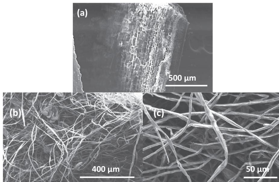
Fig. 2. SEM images of (a) raw *Juncus* stems (R-Junc) and (b) and (c) CMF.
