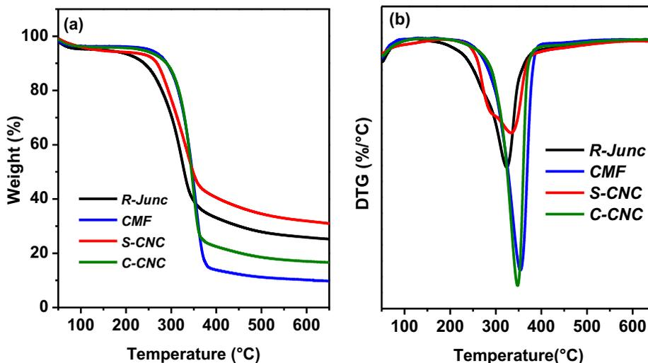
Fig.6. (a) TGA and (b) DTG curves of raw *Juncus* stems (R-Junc), CMF and CNC (S-CNC and C-CNC).
