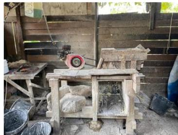
Gambar 3. Mesin Pamarut Tipe Silinder
